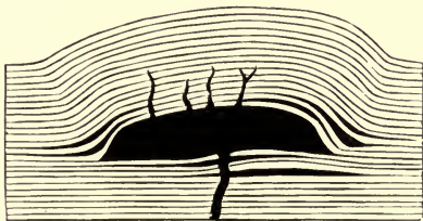
FIG. 124.—Laccolith (after GILBERT). This ideal section is drawn as if no denudation had taken place.
